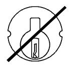
IF SHORTER OR LONGER CAMS ARE USED, THEY WILL NOT OPERATE THE MECHANISM.
