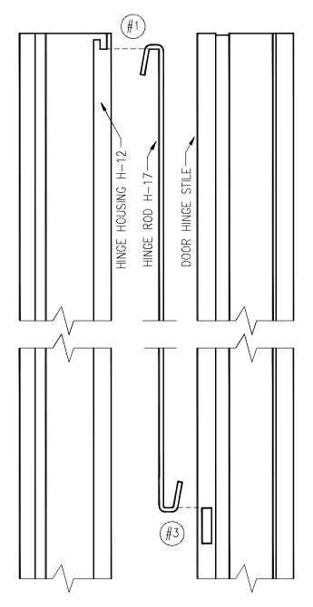
NOTE: IF REPLACING H-17 WITH H-50 HINGE HOUSING H-12 AND HINGE H-13 MUST BE REPLACED
