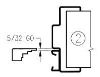
HINGE HS'G TO FRAME STOP USE 5/32 PORTION OF "KEY" TO CHÉCK FOR MINIMUM CLEAPANCE AT TOP OF JAMB.
