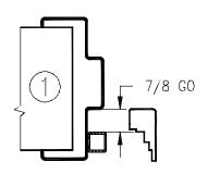
LATCH STOP TO FRAME STOP USE 7/8 PORTION OF "KEY" TO CHECK PROPER STOP POSITION
